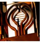
**Metal heating elements** Two metal heating elements warm up the sample.
